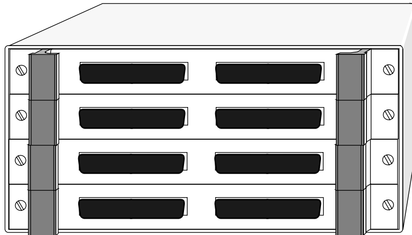
Figure 1. ENCL-4 Enclosure with Four EXP-1600s Installed
